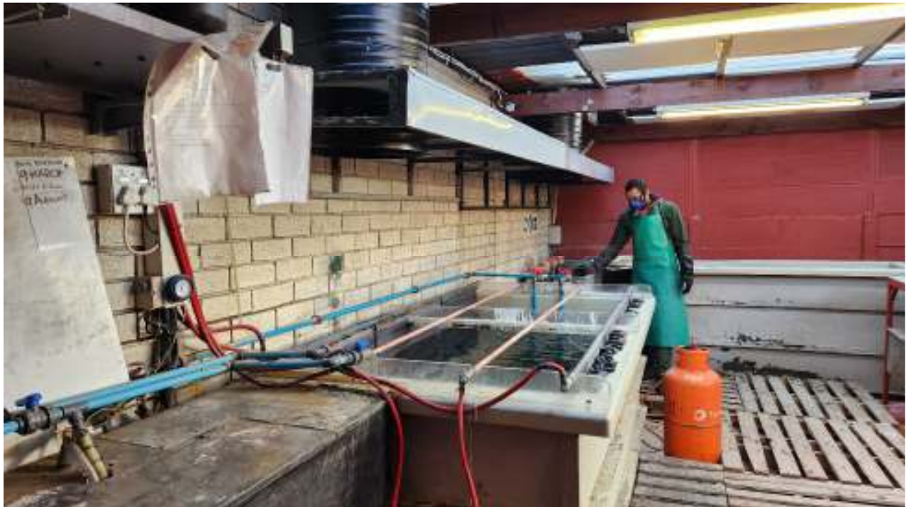
2. Chemical wash to prepare for etching
