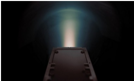
A satellite iodine electric propulsion system firing in a vacuum chamber.
