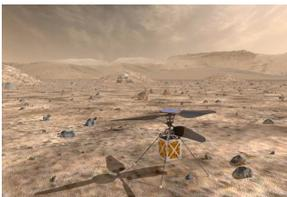
NASA's Mars Helicopter, a small, autonomous rotorcraft, will travel with the agency's Mars 2020 rover, currently scheduled to launch in July 2020, to demonstrate the viability and potential of heavier-than-air vehicles on the Red Planet. NASA/JPL-Caltech
