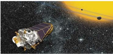
Despite losing its second of four reaction wheels in 2013, the Kepler mission continues to carry out short-term exoplanet hunting campaigns as it runs out of fuel. NASA/Kepler Mission/Wendy Stenzel
